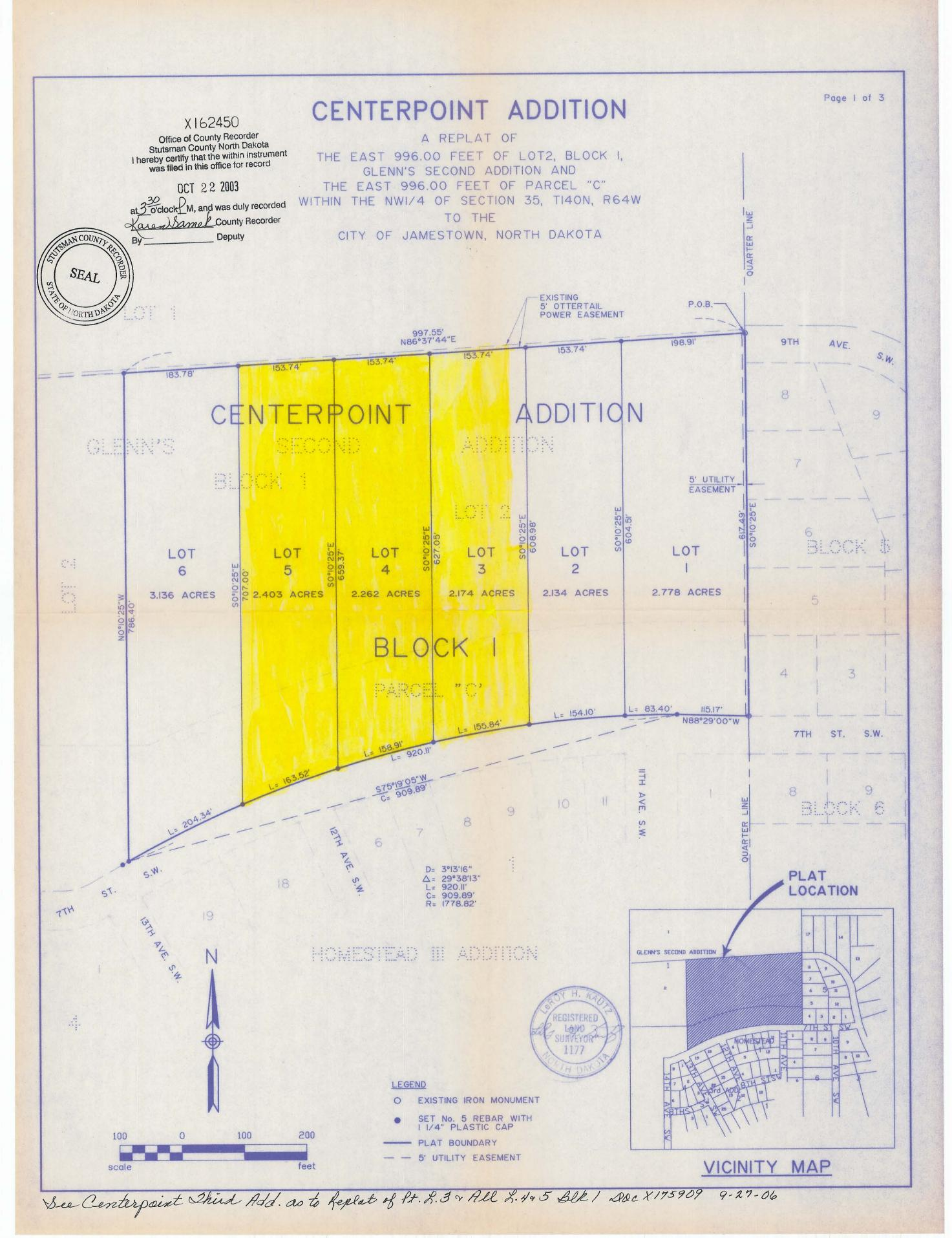
CENTERPOINT ADDITION A REPLAT OF THE EAST 996.00 FEET OF LOT 2, BLOCK I, GLENN'S SECOND ADDITION AND THE EAST 996.00 FEET OF PARCEL "C" WITHIN THE NWI/4 OF SECTION 35, TI40N, R64W TO THE
